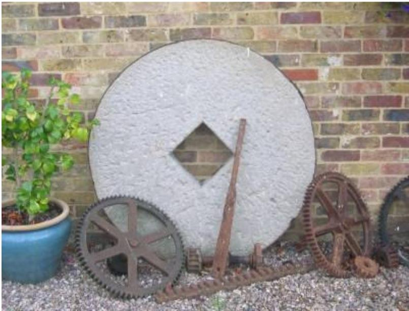
Barnes mill stones and winding gear
